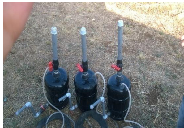
Fig. 2.1 Actual Model and Set up of Anaerobic Digester at farm
